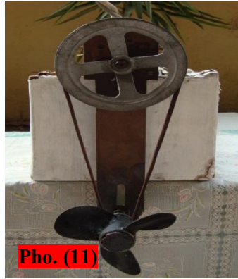
Photos 11., 12. Different views of steel frame which combines the AC motor with the propeller
