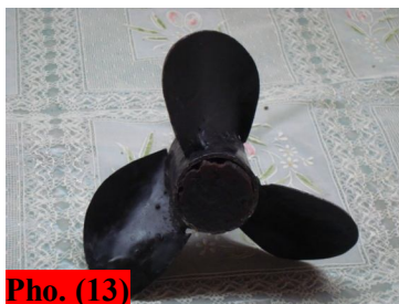
Photos 13., 14. Hollow aluminum cylinder propeller and its blades
