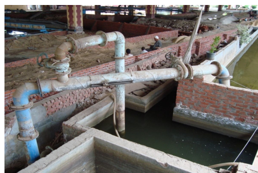
Photo 2. The main sump and the feeding system of the model intake (Front view)
