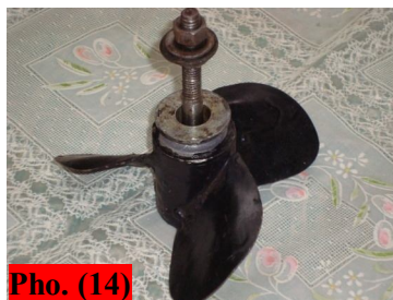
Photos 13., 14. Hollow aluminum cylinder propeller and its blades
