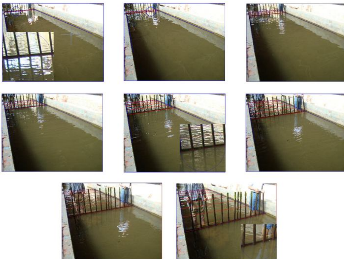
Photo 25. The contact line between both the wooden ruler and the water's surface along the longitudinal direction of the model every 1.0 m
