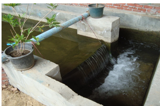
Photo 5. The outlet sump and the control gate of the model (Side view)
